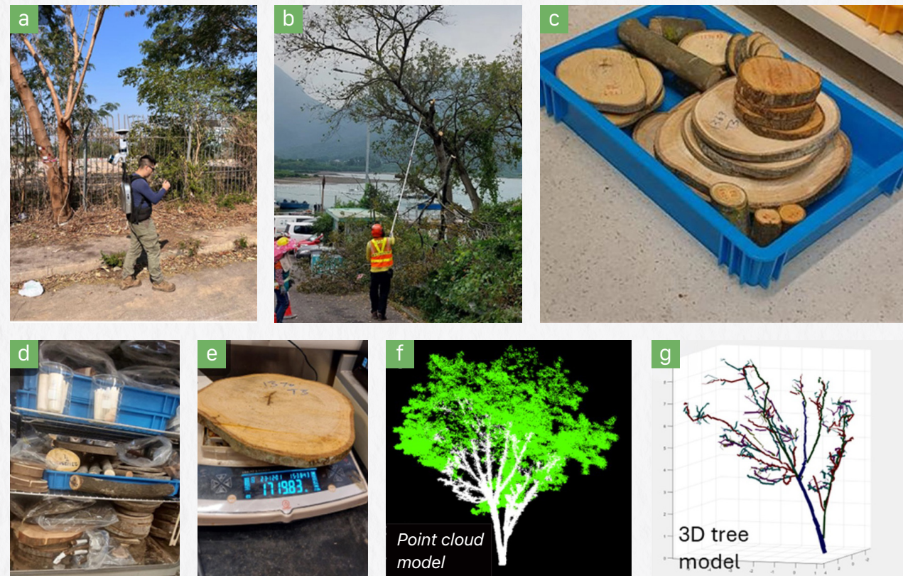
Fig. 2.1 – Field measurement and laboratory testing: (a) mobile LiDAR scanning; (b) tree felling; (c) wood samples; (d) over-drying of samples; (e) sample weighing; (f) tree point cloud model; (g) tree 3D model
